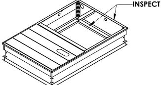
**<u>STEP 3:</u>** SET THE CURB ADAPTER DOWN ONTO EXISTING CURB ALIGNING THE SUPPLY AND RETURN AIR OPENINGS.
